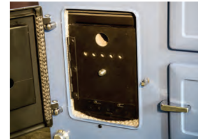
The firebox of the 905 W35 has a secondary door with peephole to check the fire and controls to adjust the burn rate
