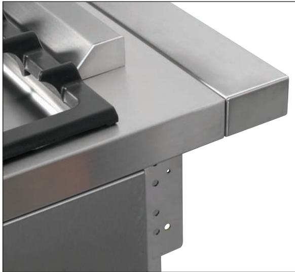
With the back infill panel in place, a 70 mm space remains between the range and the wall. The overall depth of the appliance (rail not included) then reaches 720 mm (an increase of 70 mm). The back infill panel prevents excessive heat transfer to the wall and makes cleaning easier. It is especially recommended for all ranges equipped with gas ovens or those with tiles on the wall above the cooker.
